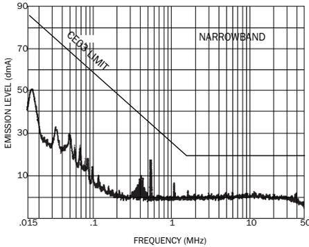
MSA2805S converter at full load with an STF28-461 EMI filter.
