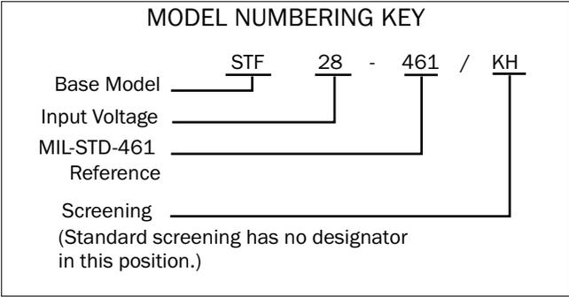
FIGURE 4: MODEL NUMBERING KEY
