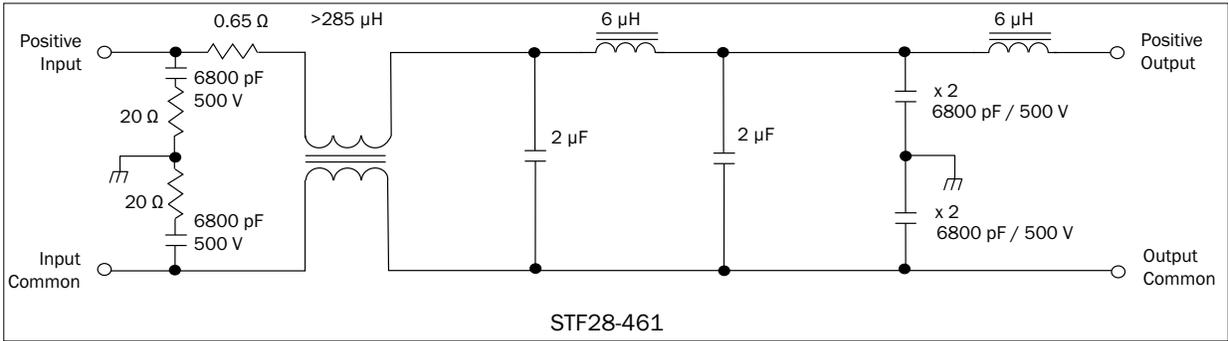
The case ground connection between the filter and the converter should be as low an impedance as possible to minimize EMI. Direct contact of baseplate to chassis ground provides the lowest impedance.
