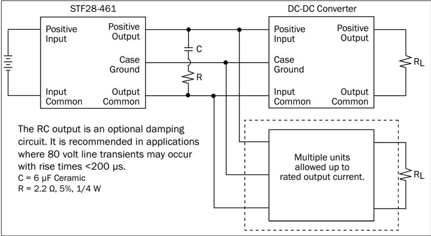
FIGURE 2: DAMPING CIRCUIT
