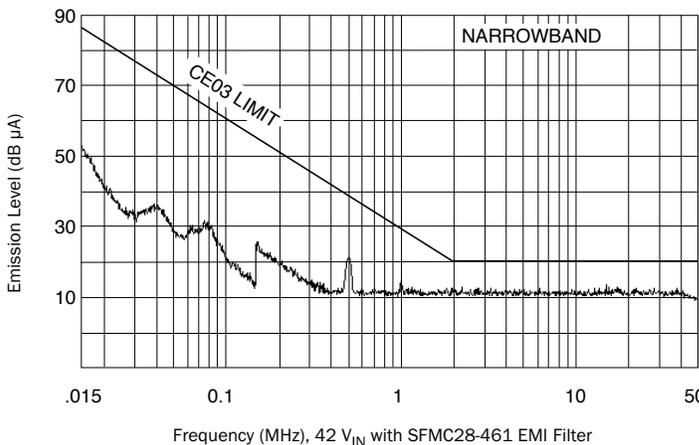
Frequency (MHz), 42 V<sub>IN</sub> with SFMC28-461 EMI Filter
