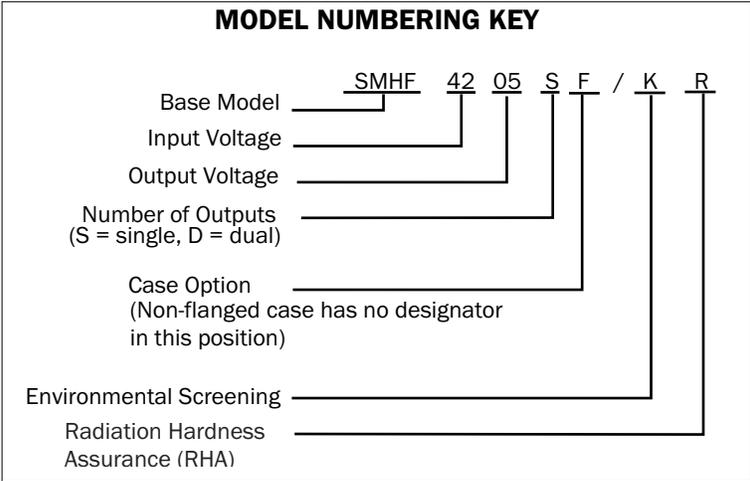
FIGURE 5: MODEL NUMBERING KEY
