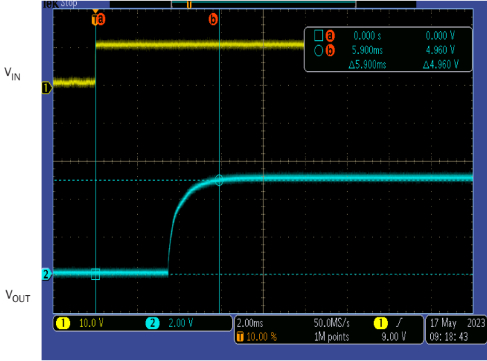
MSA+2805S START-UP RESPONSE FULL LOAD FIGURE 19
