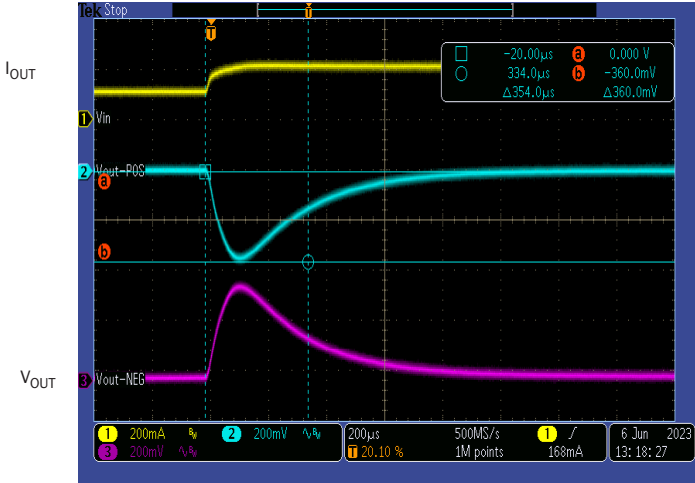
MSA+2805D STEP LOAD 50% - 100% FIGURE 28
