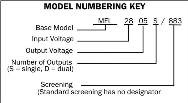
FIGURE 4: MODEL NUMBERING KEY
