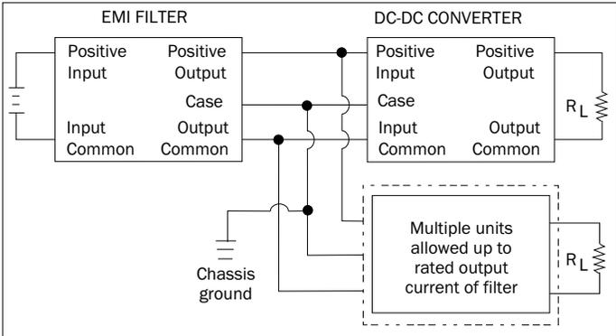
The case ground connection between the filter and the converter should be as low an impedance as possible to minimize EMI. Direct contact of baseplate to chassis ground provides the lowest impedance.
