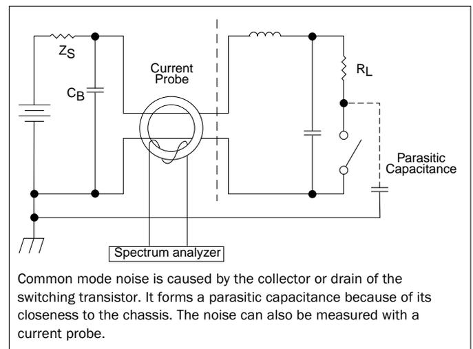
FIGURE 4: MEASURING COMMON MODE NOISE
