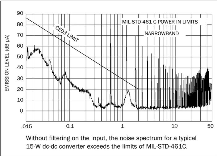
FIGURE 7: UNFILTERED DC-DC CONVERTER
