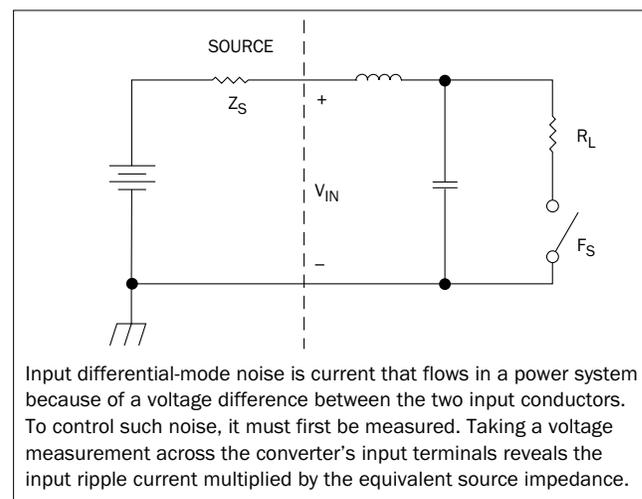
FIGURE 2: SIMPLIFIED INPUT DIFFERENTIAL MODE NOISE MEASUREMENT
