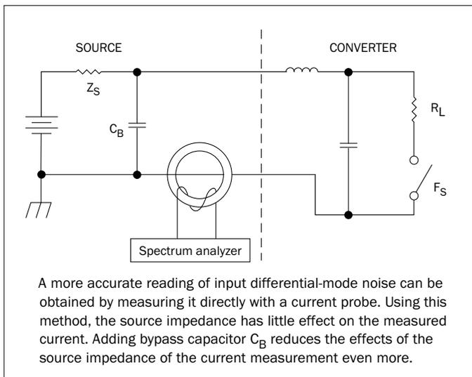
FIGURE 3: DIRECT INPUT DIFFERENTIAL MODE NOISE MEASUREMENT
