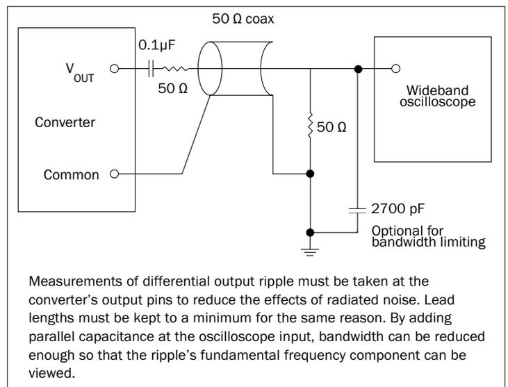
FIGURE 6: MEASURING DIFFERENTIAL OUTPUT RIPPLE
