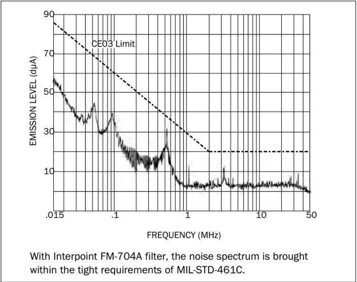
FIGURE 8: FILTERED DC-DC CONVERTER
