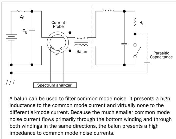
FIGURE 5: FILTERING COMMON MODE NOISE
