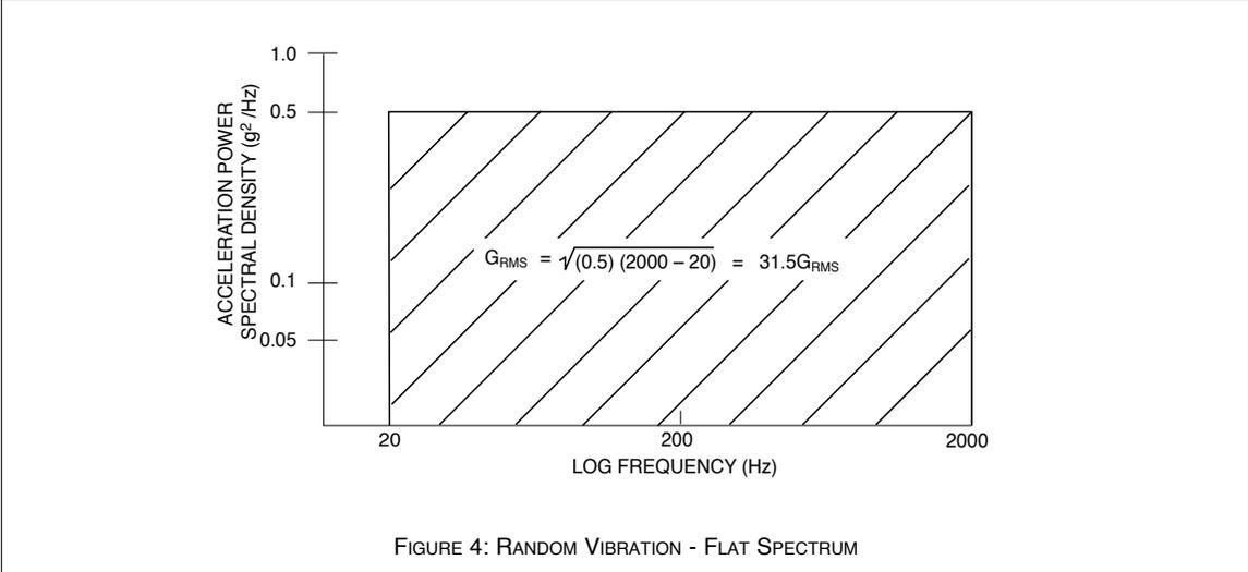
FIGURE 4: RANDOM VIBRATION - FLAT SPECTRUM
