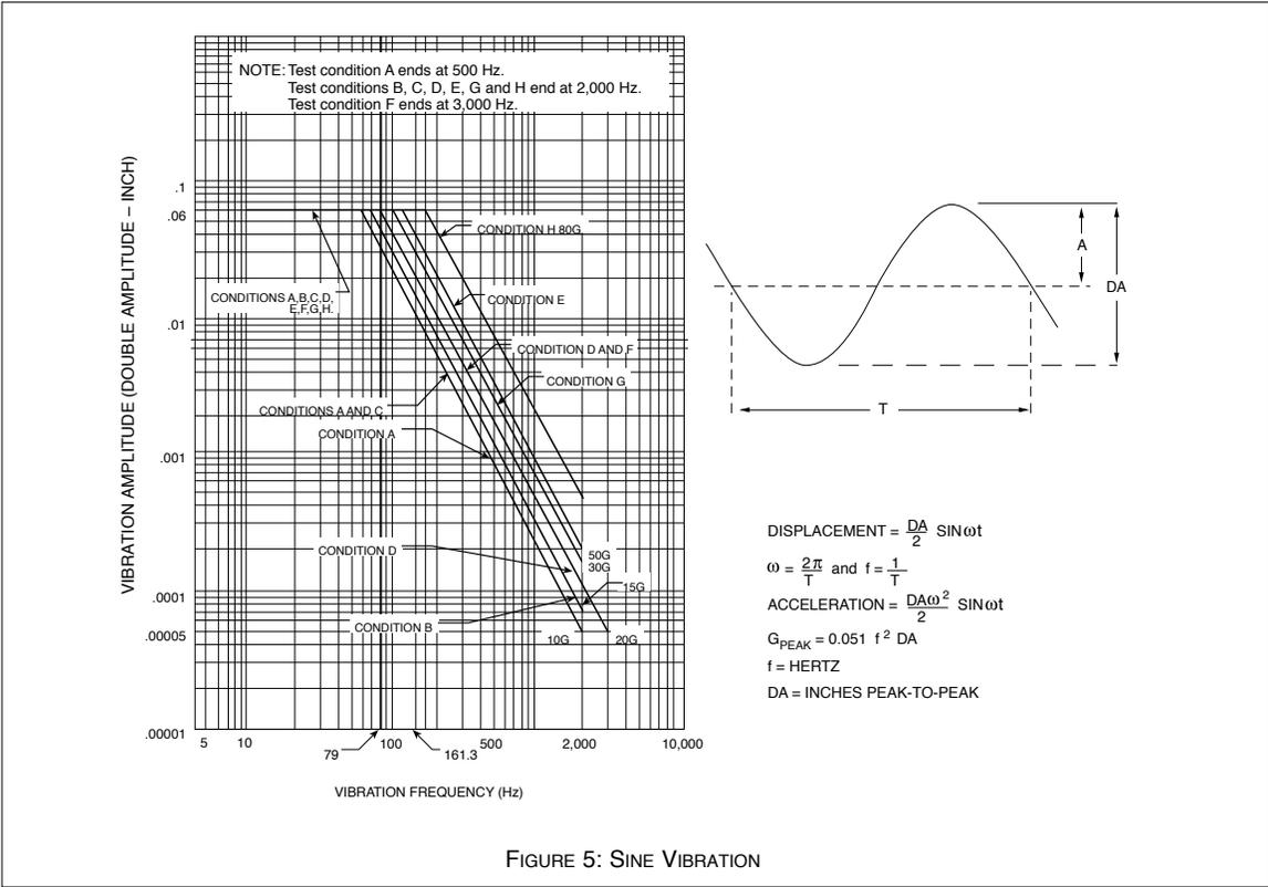
FIGURE 5: SINE VIBRATION
