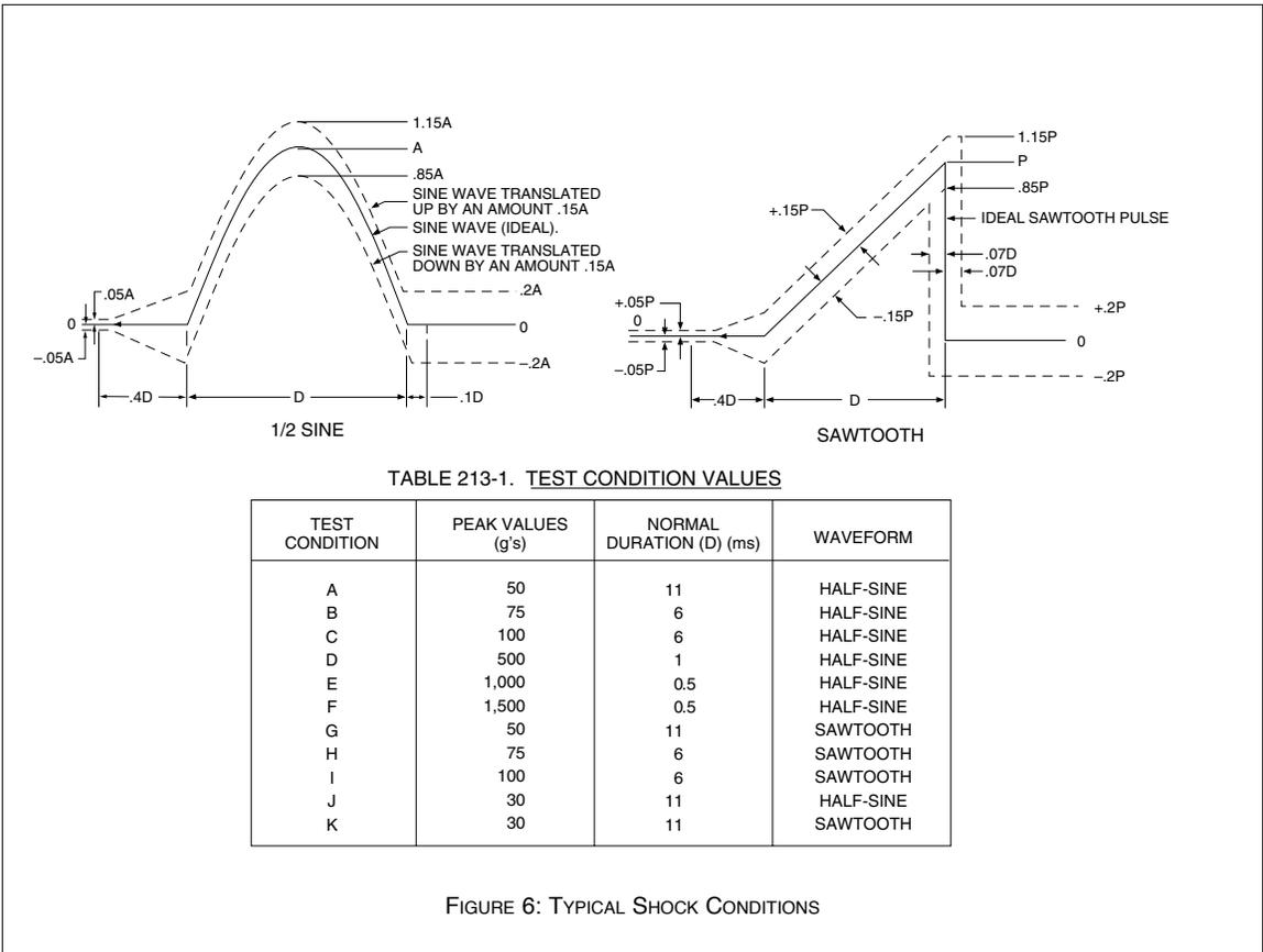
FIGURE 6: TYPICAL SHOCK CONDITIONS
