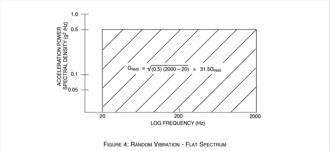
FIGURE 4: RANDOM VIBRATION - FLAT SPECTRUM
