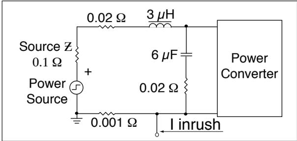
FIGURE 5: INPUT FILTER MODEL
