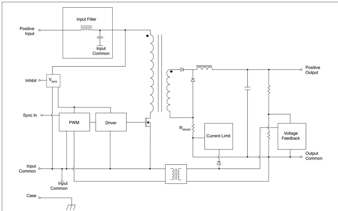
FIGURE 1: FORWARD CONVERTER WITH INPUT LINE FILTER
