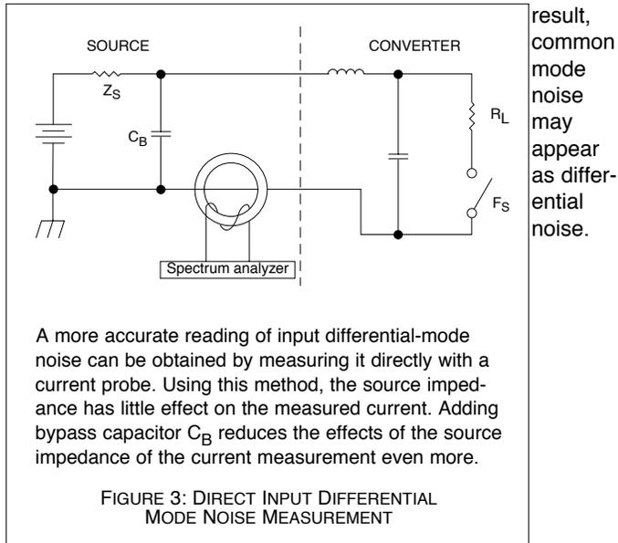
Consequently, when measuring output differential noise, it is best to connect input and output commons to case, and to use the case as a single point ground for all test equipment to minimize common mode interference.
