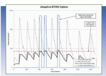
The output of the new **Adaptive BTMS** (a feature of the Tire Pressure and Brake Temperature Monitoring System, available for the 737 MAX aircraft) indicates only three dispatch delays are required for the same flight profile. A more accurate prediction of fuse temperature is enabled through the use of two temperature measurement points.
