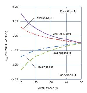
CONDITION A LOAD: -V 50%, +V 50% TO 10% CONDITION B LOAD: +V 50%, -V 50% TO 10% CROSS REGULATION
