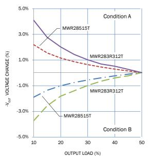
CONDITION A LOAD: -V 50%, +V 50% TO 10% CONDITION B LOAD: +V 50%, -V 50% TO 10% CROSS REGULATION
