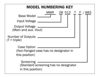
FIGURE 3: MODEL NUMBERING KEY
