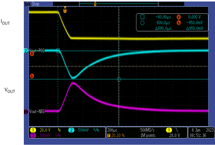
UNITS ARE PER DIVISION MSA+2805D STEP LINE 50 - 15V FULL LOAD FIGURE 31
