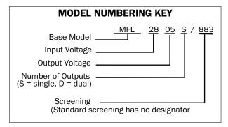
FIGURE 4: MODEL NUMBERING KEY
