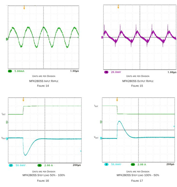
$\label{eq:typical performance Plots: 25 °C case, 28 Vin, 100\% \ \mbox{load, unless otherwise specified.} \\ For reference only, not guaranteed specifications. \\$
