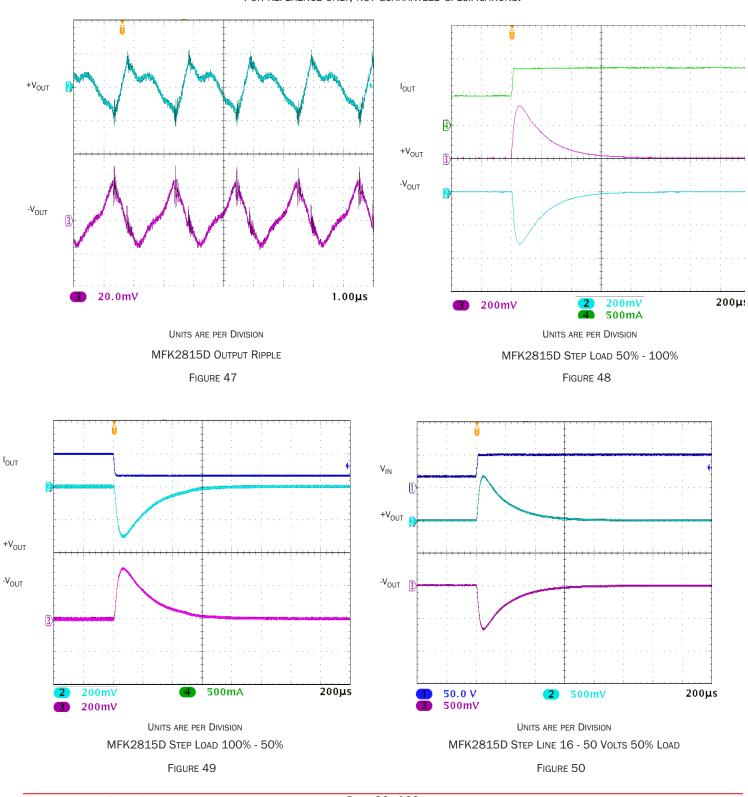
Typical Performance Plots: 25 °C case, 42 Vin, 100% load, unless otherwise specified. For reference only, not guaranteed specifications.
