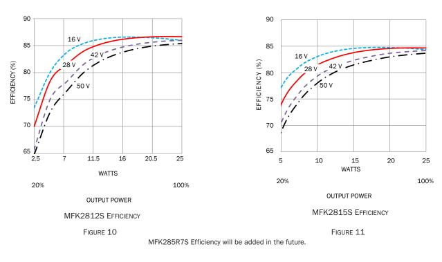
Typical Performance Plots: 25 °C case, 28 Vin, 100% load, unless otherwise specified. For reference only, not guaranteed specifications.
