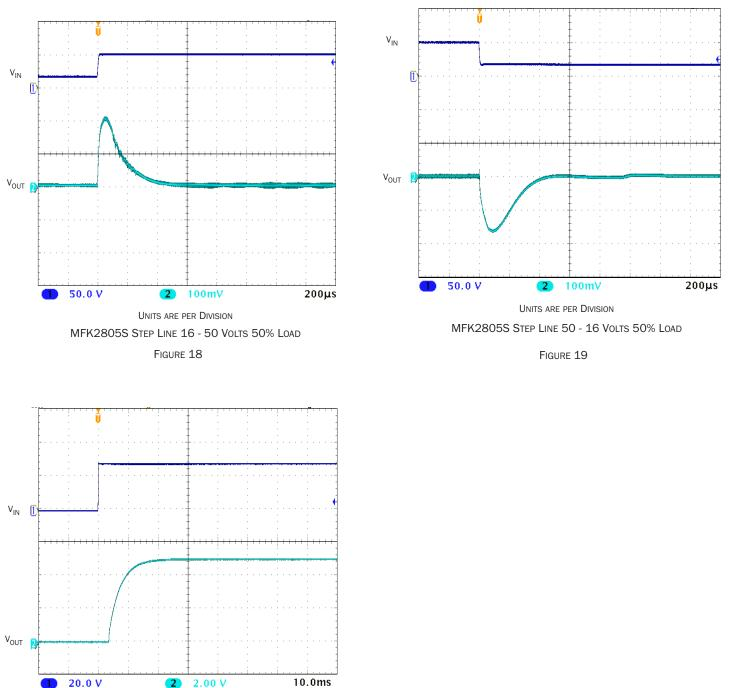
Typical Performance Plots: 25 °C case, 28 Vin, 100% load, unless otherwise specified. For reference only, not guaranteed specifications.
