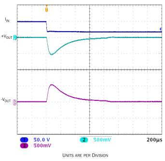
MFK2815D STEP LINE 50 - 16 VOLTS 50% LOAD
