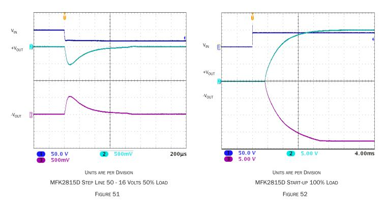
Typical Performance Plots: 25 °C case, 42 Vin, 100% load, unless otherwise specified. For reference only, not guaranteed specifications.
