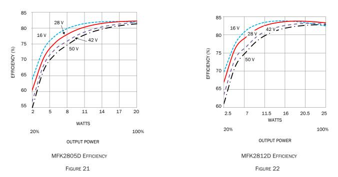
$\label{eq:typical performance Plots: 25 °C case, 28 Vin, 100\% \ \mbox{load, unless otherwise specified.} \\ For reference only, not guaranteed specifications.$
