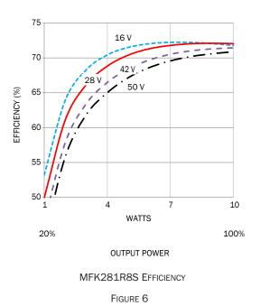
Typical Performance Plots: 25 °C case, 28 Vin, 100% load, unless otherwise specified. For reference only, not guaranteed specifications.
