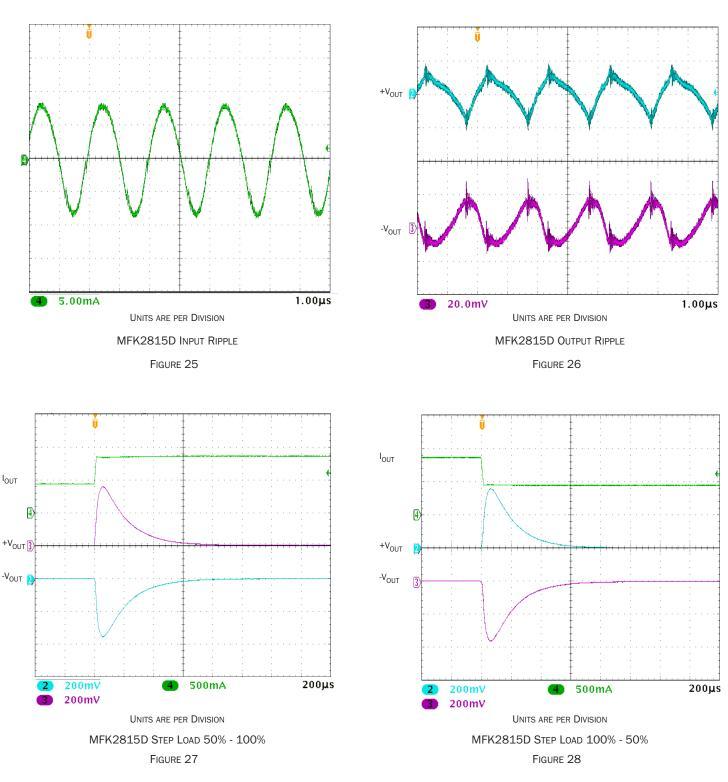
Typical Performance Plots: 25 °C case, 28 Vin, 100% load, unless otherwise specified. For reference only, not guaranteed specifications.
