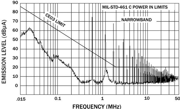
DC-DC CONVERTER AT FULL LOAD TYPICAL
