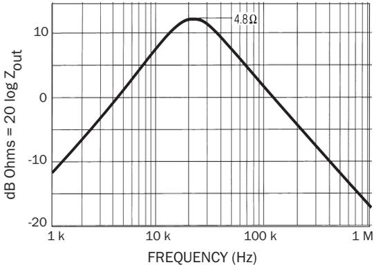
TYPICAL OUTPUT IMPEDANCE (Z) WITH INPUT SHORTED
