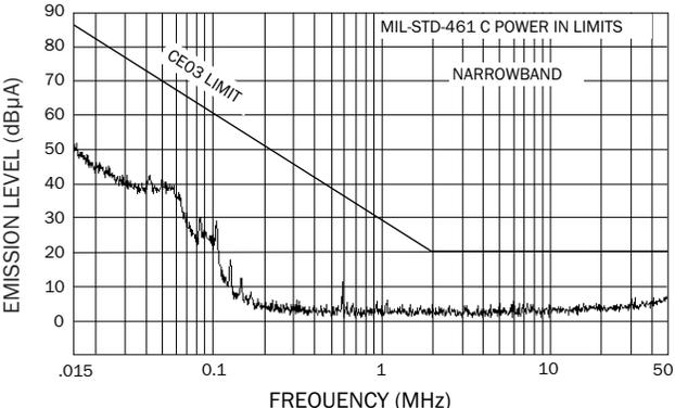
DC-DC CONVERTER AT FULL LOAD TYPICAL
