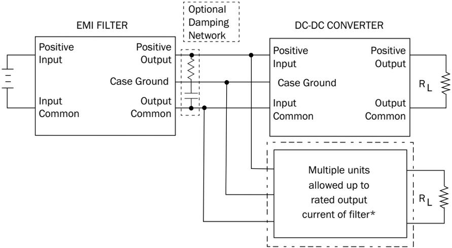
FIGURE 2: CONNECTION DIAGRAM
