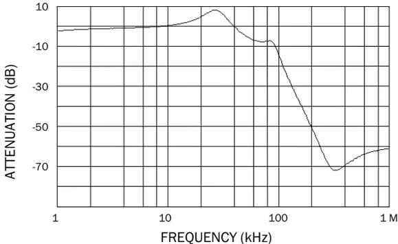
FMC-461 TYPICAL AMPLITUDE RESPONSE VS. FREQUENCY
