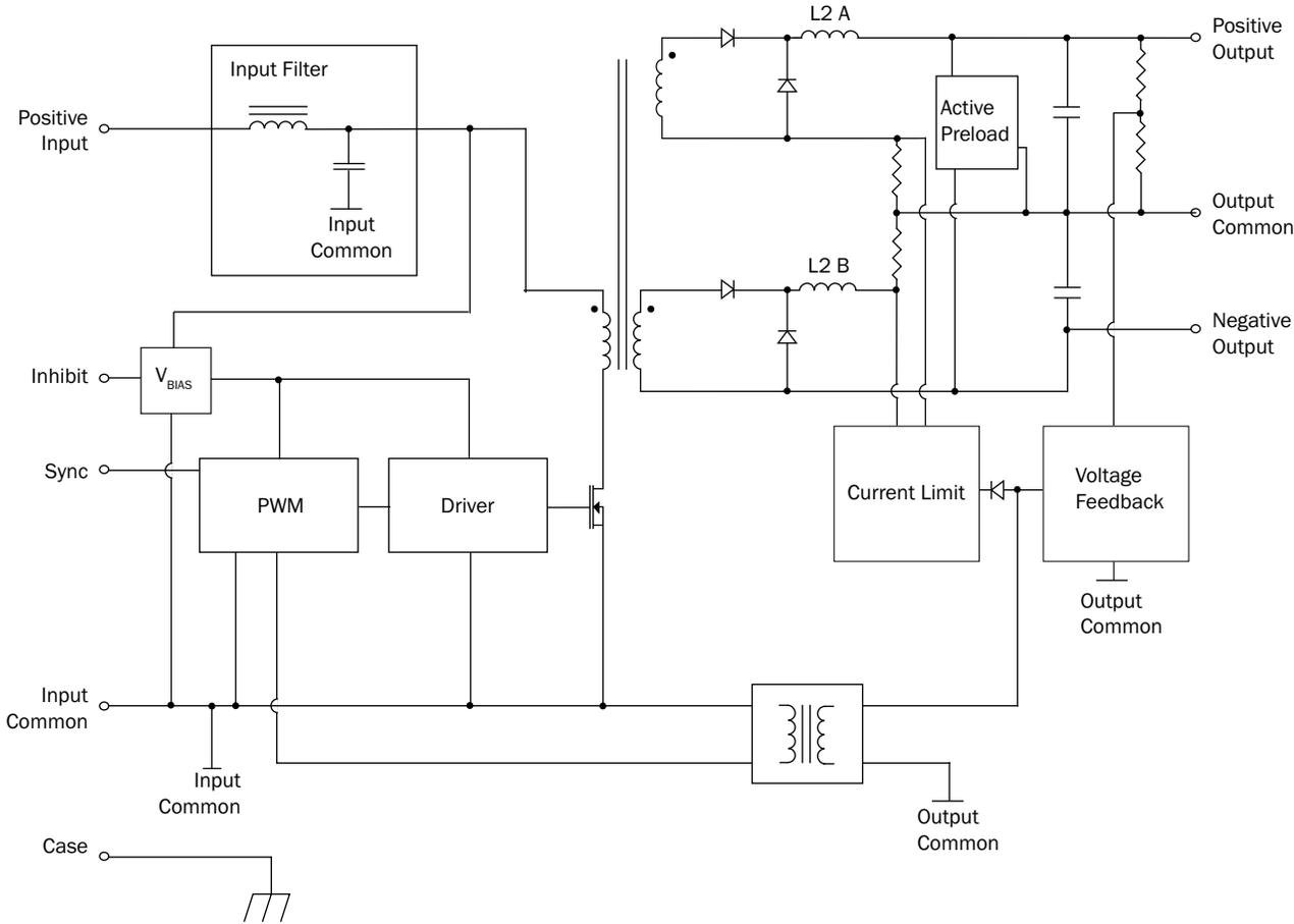
FIGURE 3: MTR DUAL NON-883 BLOCK DIAGRAM
