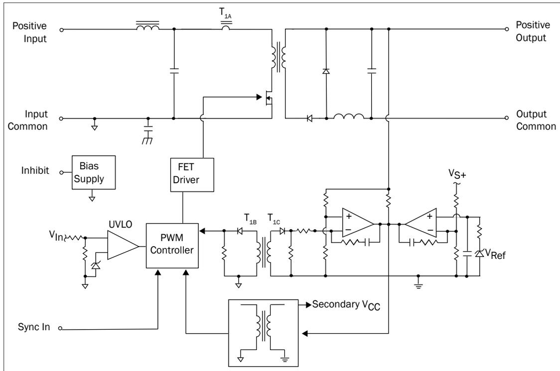
FIGURE 1: MFK SINGLE BLOCK DIAGRAM
