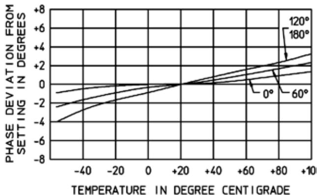
Figure 6: Typical Phase vs. Temperature
