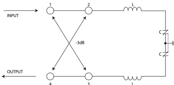
Figure 1: Mechanical Phase Shifter Section
