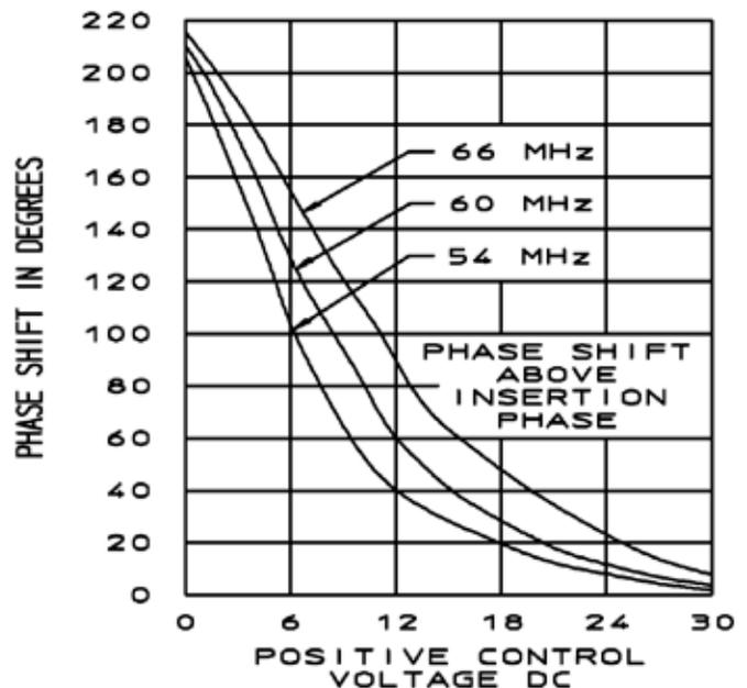
Figure 4: Typical Phase Shift vs. Control Voltage
