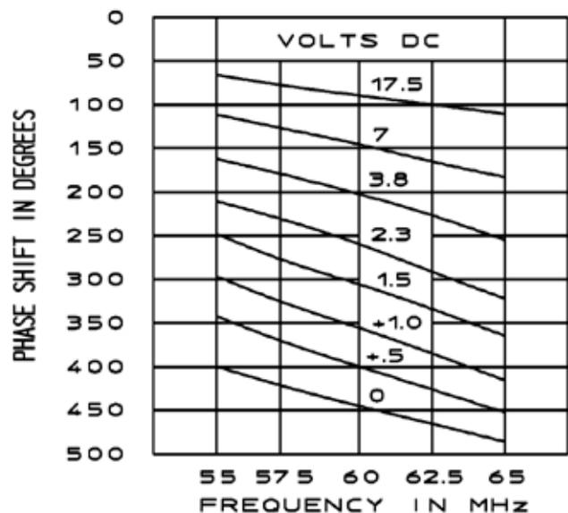
Figure 5: Typical Phase Shift vs. Frequency
