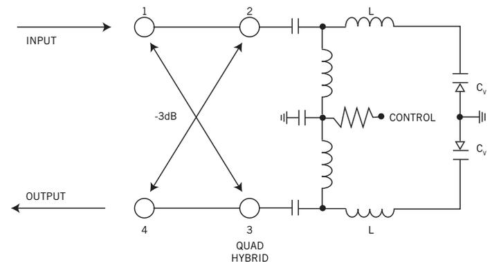
Figure 2: Electronic Phase Shifter Section
