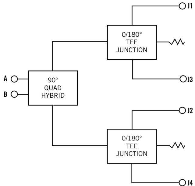
**Figure 2: Quadrapole Network Schematic**
