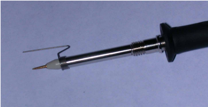
FIGURE 8: PIG-TAIL USED IN FIGURE 9 MEASUREMENT
