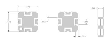
NOTES: Dimensional tolerance unless otherwise specified shall be: +/-.005" Thickness tolerance: +/-.005"
